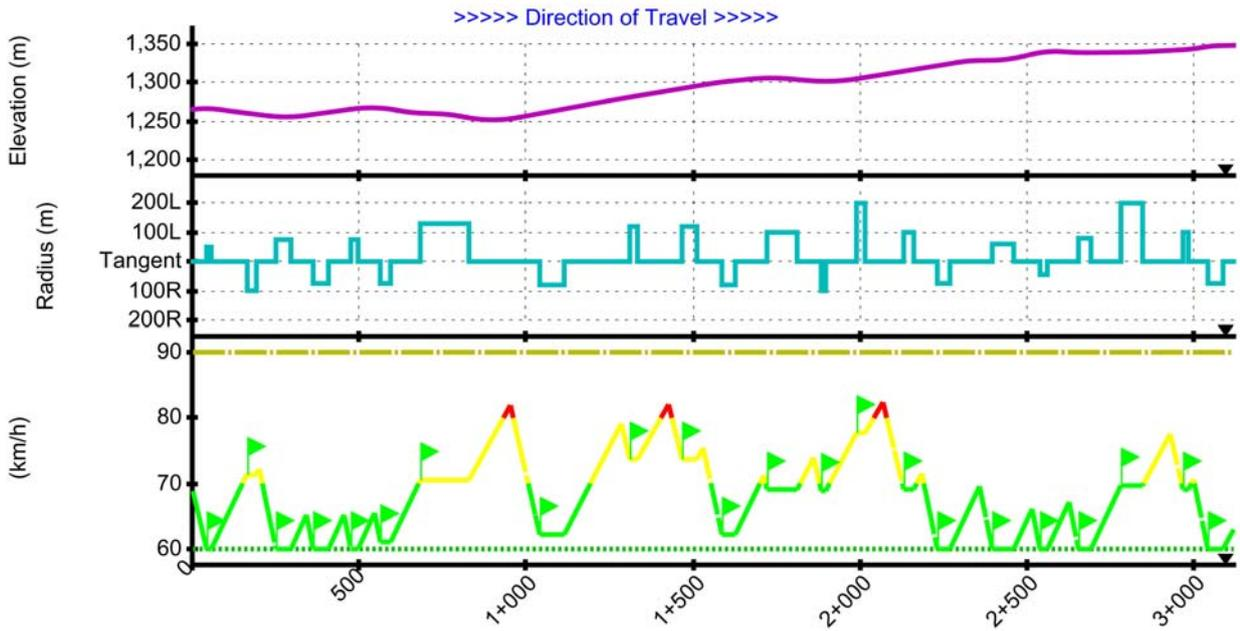
Fig. 4 IHSDM – Design consistency analyze of test section
