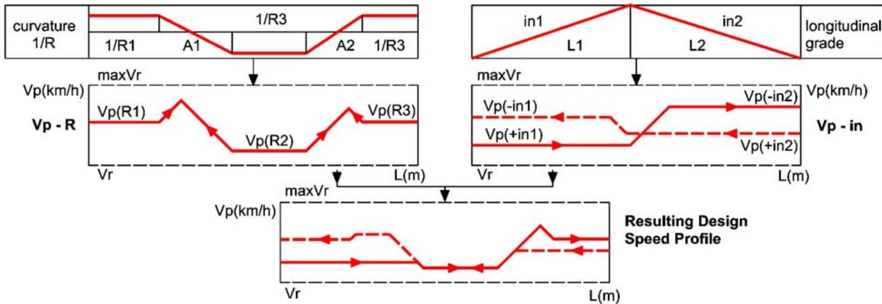
Fig. 2 Development of the resulting design speed profile
