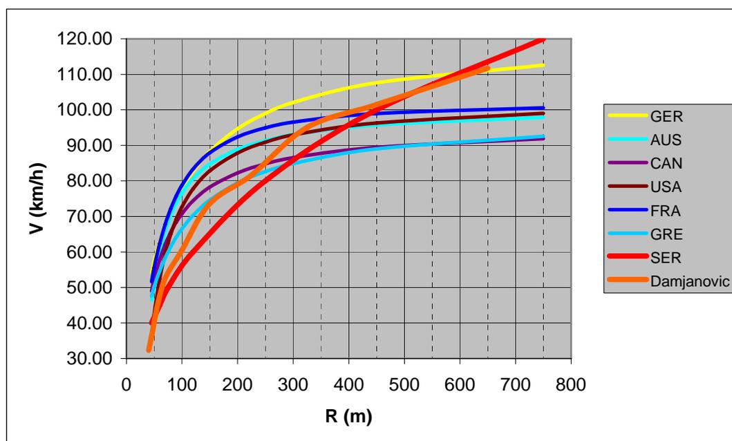
Fig. 3 Diagram showing dependence of the 85<sup>th</sup> percentile speed on horizontal radii
