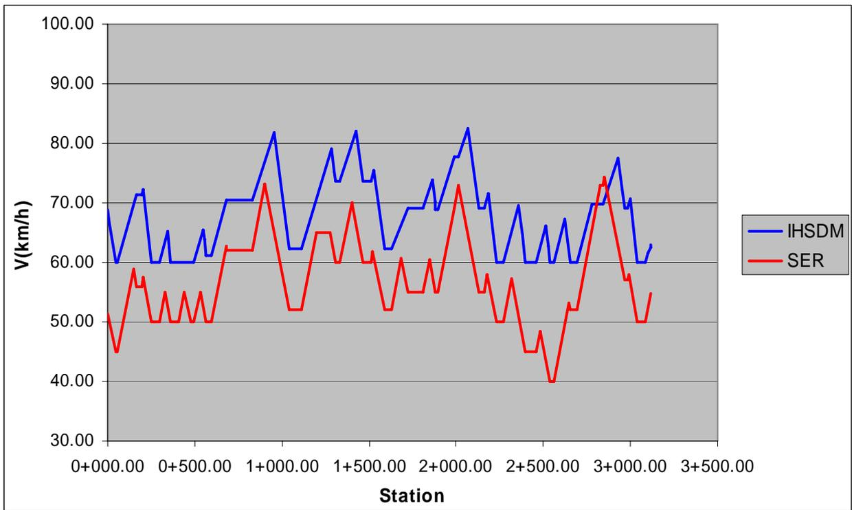
Fig. 5 Comparison between IHSDM speed model and presented speed model
