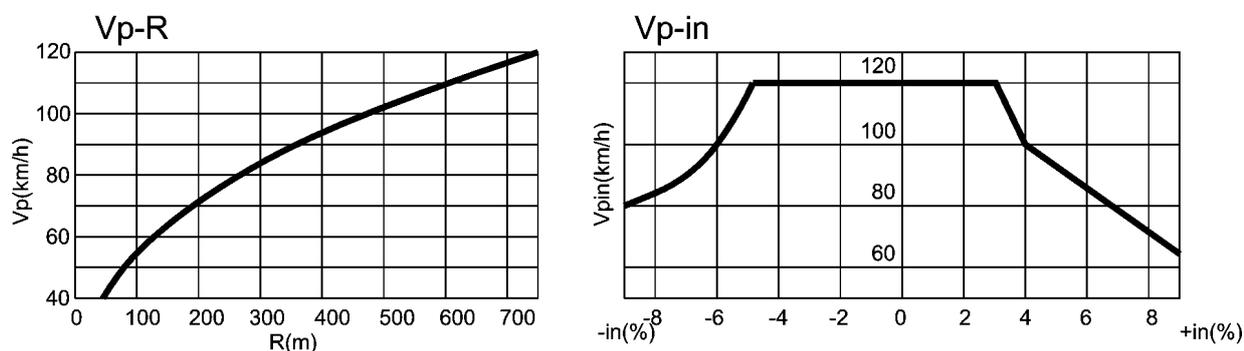
Fig. 1 Dependence: vehicle speed – radius and vehicle speed - longitudinal gradient
